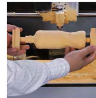
Once MODELA has finished milling, remove the part from the supports that secured the material to the unit and file the cut surfaces away.
