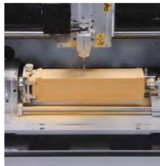
Once you finish attaching the milling cutter and positioning the material, close the cover. You are now ready to start milling. Select the Start Cutting button on your screen and the MDX will begin milling.
