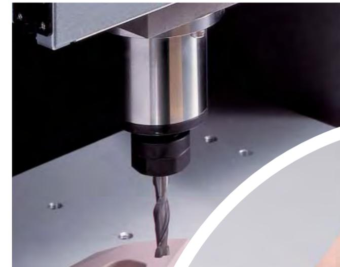
Prototyping is critical to the product development process, allowing designers to both see and touch the results of their work. With a prototype, designers can review their designs at every angle and assess many attributes not reflected in printed designs or on screen — including the precise size, surface finish and ease of manufacturing of a design. Roland MODELA series 3D milling machines produce precision prototypes quickly and easily, making them ideal for in-house designing.
