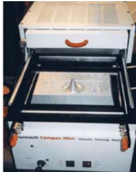
Fig. 5.4 A Metapor mould demonstrated on one of the Formech range of vacuum forming machines
